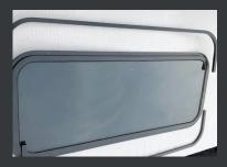
Take the frame from the kit and place in the hole to check fit as they are made to be tight fit, you made need to file where the screws join the frame together once your happy remove the frame now take the glue and with precut nozzle apply even glue bead around the edge of the frame and then place in hole
