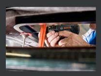
we leave fixing of frame up to customer you can use self tapping screws or pop rivets fix in finishing frames and inner trims can be refitted at this point too
