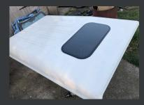
Now your ready to fit roof glass with a new wipe clean and dry glass edge and inner frame then as before prime the glass and frame let this dry for 5mins apply an even bead of glue round inner frame and fit glass clean any excess of the inside you can fill frame to glass if you wish but its not necessary
